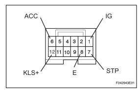
(b) Using an ohmmeter, measure the resistance at terminal E (8) and body ground.
